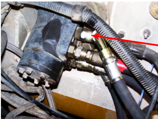
Figure 1-9: Mounting The Counterbalance Valve
