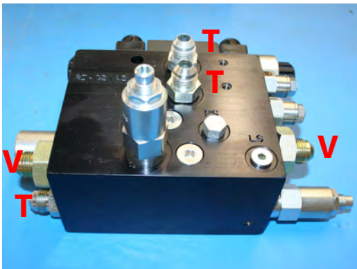
Figure 1-2: Preparing Hydraulic Control Block
